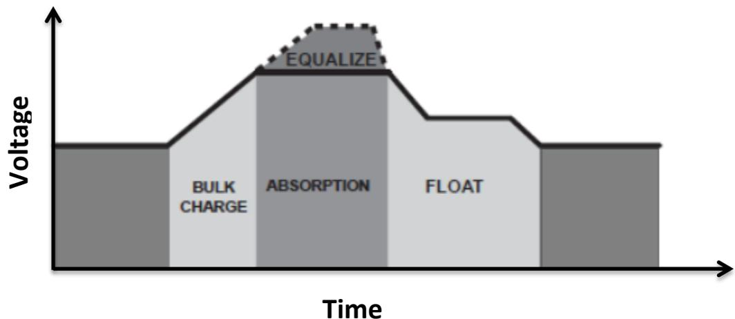
Figure 3: Battery Charging Profile
