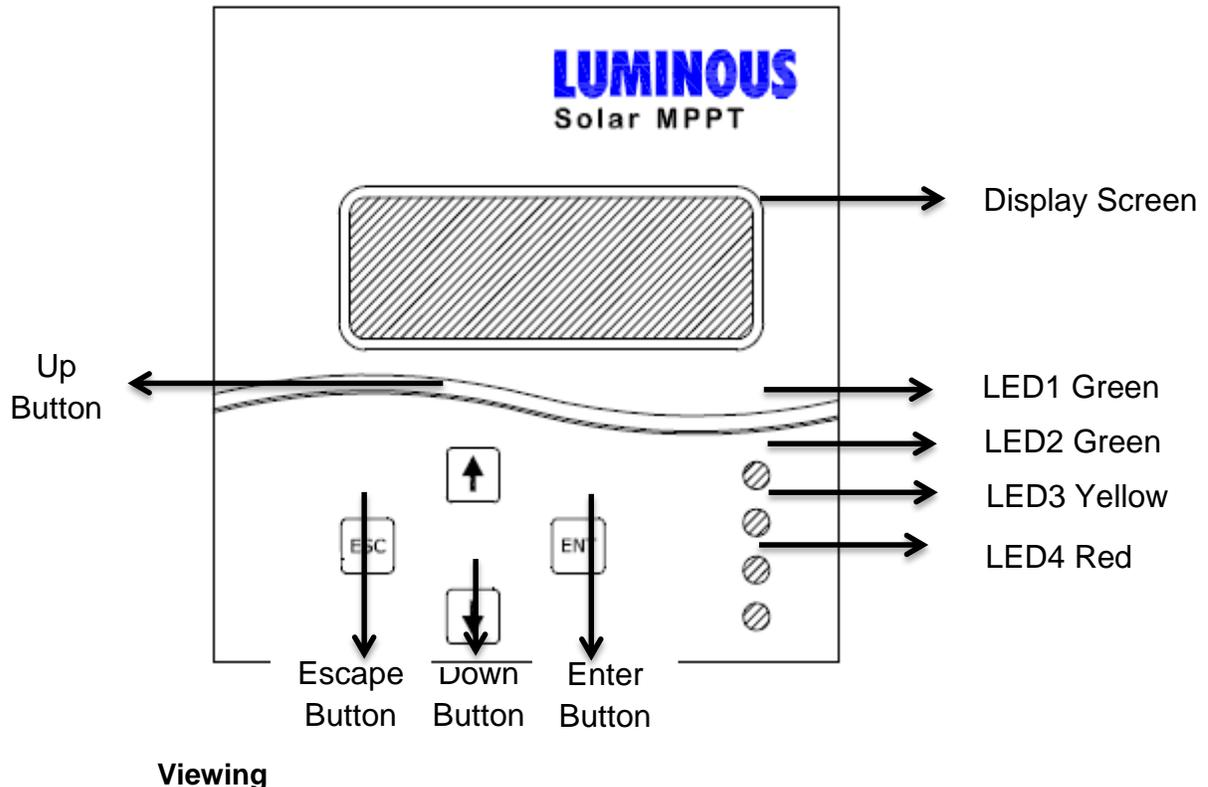
The Solar MPPT 60 has 20 character and 4 line LCD display for displaying system information and operation.
