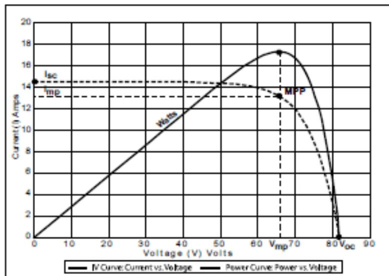
Figure1: Maximum Power Point Curve
