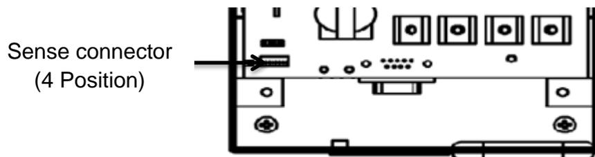
There is DB9 connector for communication wiring viz. P1. It is used for communicating with the personal computer.
